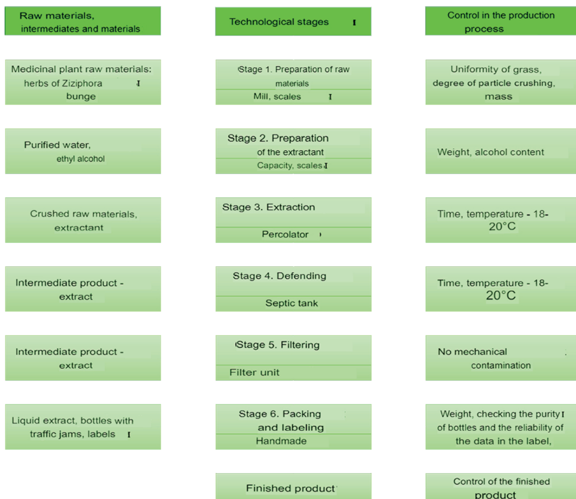
Figure 1 - Technological scheme for obtaining a liquid extract of Ziziphora bungeana Juz.
