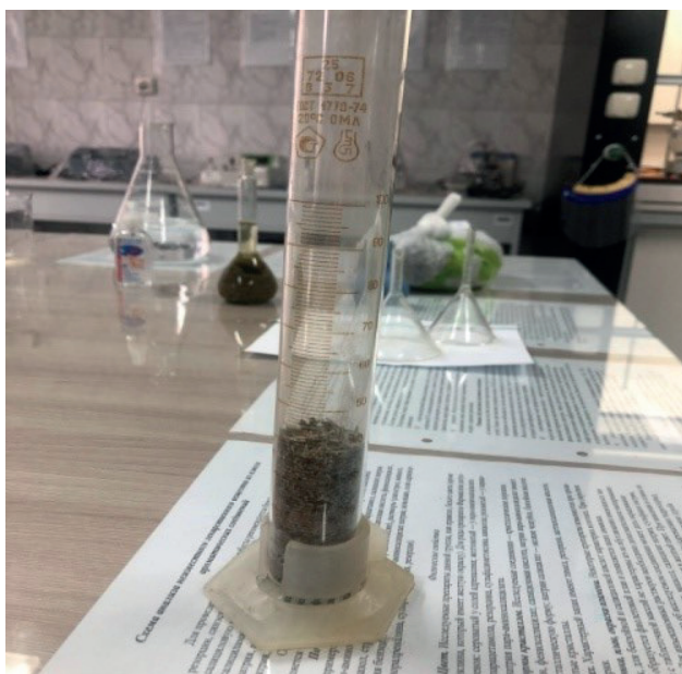
Figure 3 – raw material 10.0 g (exact weight) placed in the cylinder
